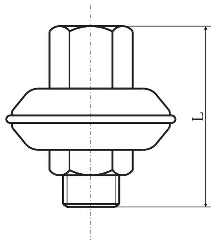
TKZ's housing is not retractable so it is not foreseen the possibility of replacing capsule.
